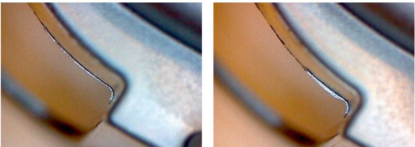
Fig. 6. The flash height of the injection molded parts depends directly on the flow behavior of the melt, and therefore on its viscosity. The Fillcontrol system determines and regulates, e.g., the viscosity of the melt in the form of shear rate and shear stress, resulting in the flash height of the parts. In the figure at the right-hand side, significantly higher flash can be seen because of a lower melt viscosity
