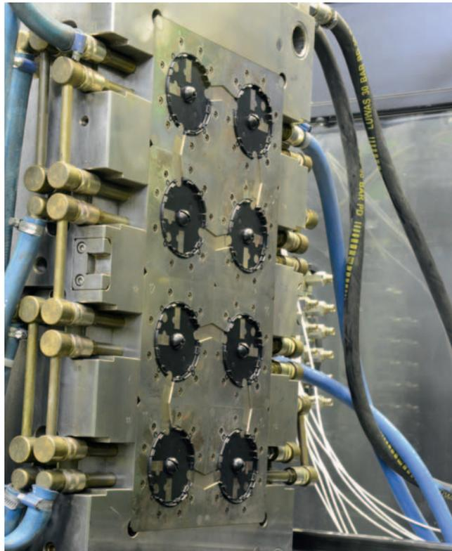
**Fig. 1. Eight-cavity hot-runner mold for manufacturing base plates for adjustment motors of side mirrors. For automatic hot-runner balancing a temperature sensor is incorporated into each cavity, and a pressure sensor is additionally incorporated into one cavity for quality control**
