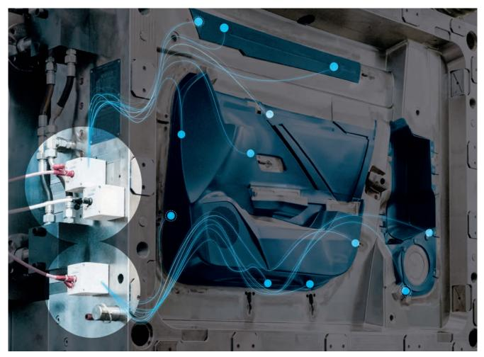
Priamus control technology enables automatic cascade adjustment and simplifies set-up. © Priamus / Barnes Molding Solutions
