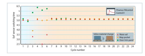
**Fig. 5.** Automatic compensation of fluctuations in the material properties on the example of the inline change to recompound.
