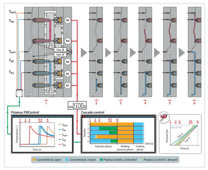
**Fig. 1.** Automatic cascade control using temperature sensors and Priamus Fillcontrol Switch. The family mold shown here has two different cavities and a total of five valve gate nozzles (N1-N5). The different colors of the compound (blue and red) identify the different molded parts. © Priamus / Barnes Molding Solutions
